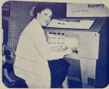
Miss Jean Warwick, assembling miniature ball bearings inside the De Luxe Model of the Pressurized Assembly Cabinet which was exhibited on our Stand at the B.I.F., Birmingham
