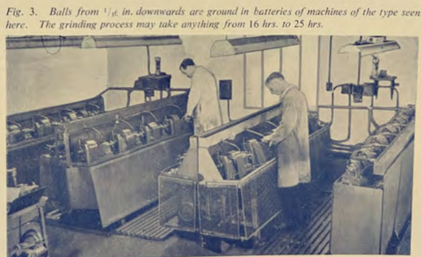
Fig. 3. Balls from 1/4 in. downwards are ground in batteries of machines of the type seen here. The grinding process may take anything from 16 hrs. to 25 hrs.
